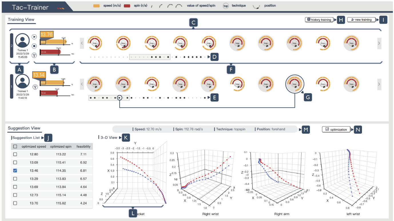
Fig. 6. The interface of Tac-Trainer for table tennis. The system contains two views, a training view, and a suggestion view. The training view visualizes the strokes in a training session through a customized flow (C) consisting of a metadata panel (A), a control panel (B), and a stroke flow (F). The suggestion view provides a list of optimization suggestions (J) for a poorly-performed stroke (G). Each suggestion can be explored in a 3-D coordinate (K). The interface presents the details of Case 1. E is the first training session and D is the second. G is the stroke chosen for optimization. L is the optimization suggestion chosen by the coach.
